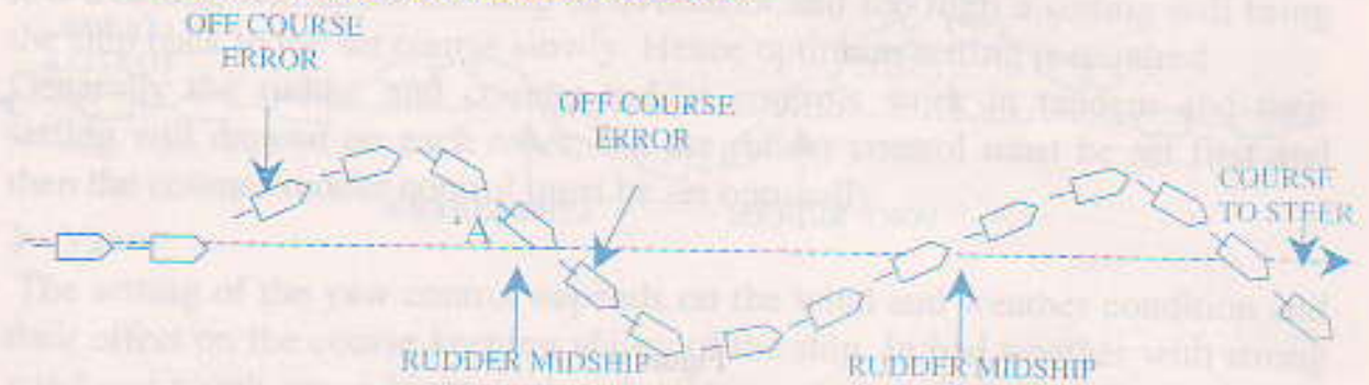
Figure 2 Motion of the ship due to proportional control only
