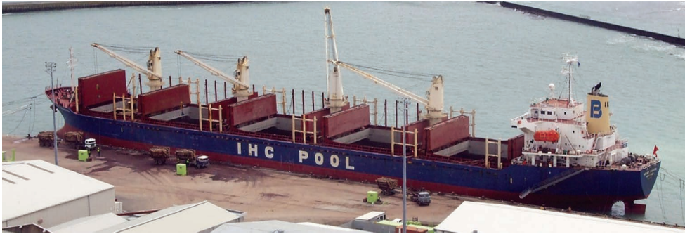
FIGURE 7.5 A vessel loads short timber logs from quayside trailers to cargo holds. The uprights are identified for the purpose of securing lashings for any timber deck cargo.
