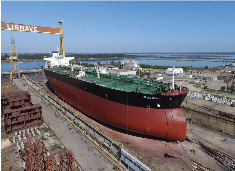
FIGURE 6.6 The Seoul Spirit (IMO No. 9248409) VLCC tanker seen in the Lisnave shipyard and dry docking complex in Portugal following hull coating and general maintenance.
