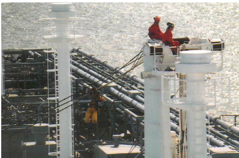
FIGURE 1.13 On-going maintenance of topping lifts, of derricks aboard a tanker vessel. Tankers generally have either derricks or cranes in an amidships position to lift pipe line connections on board close to the manifold. The derrick systems are usually supported by 'Samson posts' to accommodate tank venting and upper block securings.
