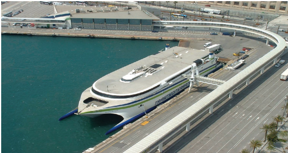
FIGURE 8.33 The High-speed RoPax Catamaran vessel Millennium Dos (IMO No. 9237644) seen loading vehicles via the stern access, lying port side to the terminal in Barcelona, Spain.
