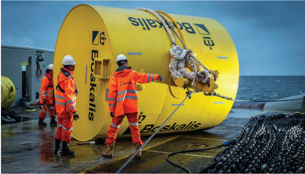
FIGURE 13.10 Offshore anchor buoys employed to locate and recover anchors to the deck of anchor handling vessels. Offshore installations (non-permanent) are often positioned amidst a pattern of anchors. Depending on size and nature of work, 8, 10 or 12 anchors would not be considered abnormal. Each anchor would be identified and marked by a recovery buoy and suitable riser.
