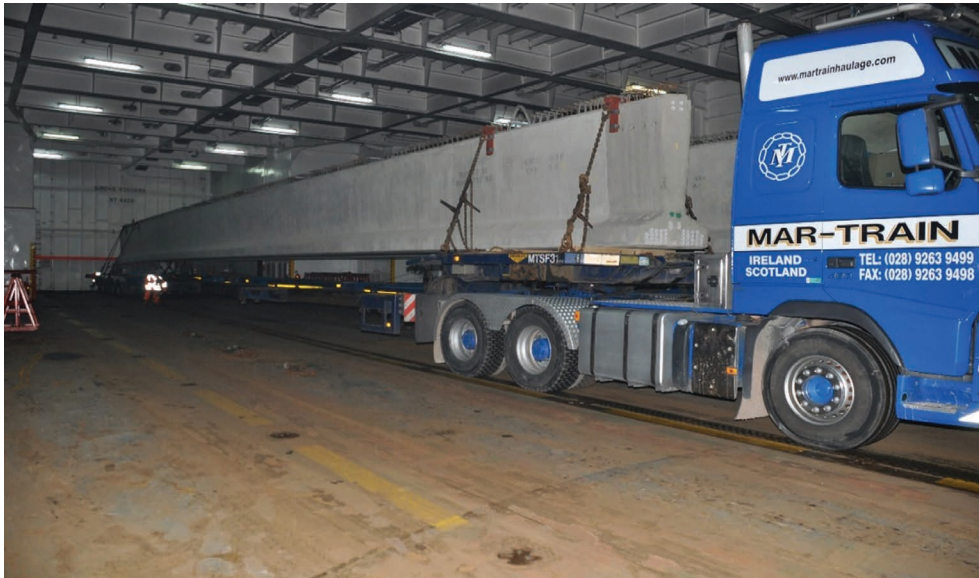
FIGURE 8.21 Long load seen on the main vehicle deck after the vehicle lashings have been removed and the unit is ready to discharge from the ferry Clipper Point .
