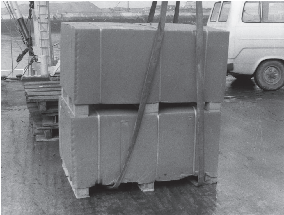
FIGURE 1.25 Canvas and nylon straps are more frequently employed with soft package materials like cardboard cartons. The straps are user friendly, strong and pliable, and cause limited damage.
