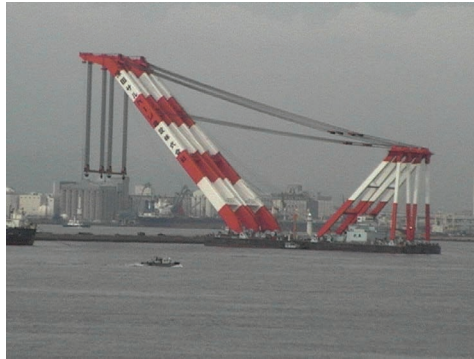
FIGURE 4.18 Heavy lift 'Sheer Leg' platform the 'Musashi' floating crane barge, seen off Kobe, Japan. This barge platform is towed to its working position. It has excessive ballast capacity for making extreme lifts up to 3,700 tonnes.
