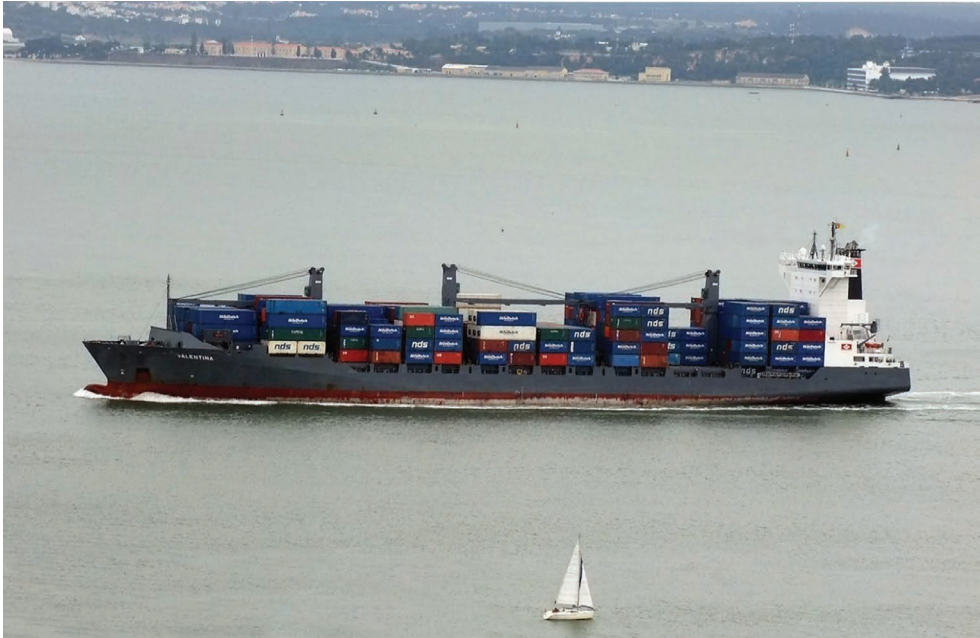
FIGURE 9.8 The container vessel Valentina (IMO No. 9344722) seen loaded in a seagoing condition. The ship is equipped with its own container cranes.
