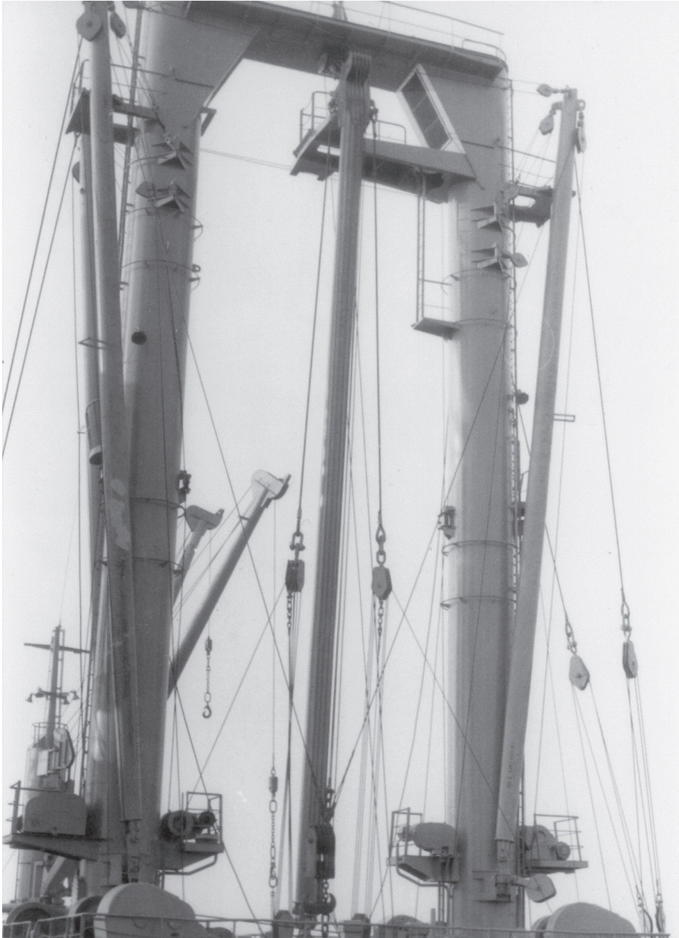
FIGURE 4.3 Conventional Jumbo heavy lifting derrick, seen in the vertically stowed position clamped to a double Samson Post (goal post) structure. The Samson posts also support smaller 10 tonne S.W.L. derricks for working general cargoes other than heavy lifts.
