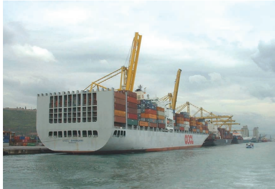
FIGURE 9.18 The OOCL Shanghai (IMO No. 9198111) lies port side to the container terminal in Barcelona, Spain, after completing cargo loading with a full container load. The deck stack is at a six tier height. The terminal gantry cranes are seen in the upright and clear position. (The ship is not fitted with its own crange.)
