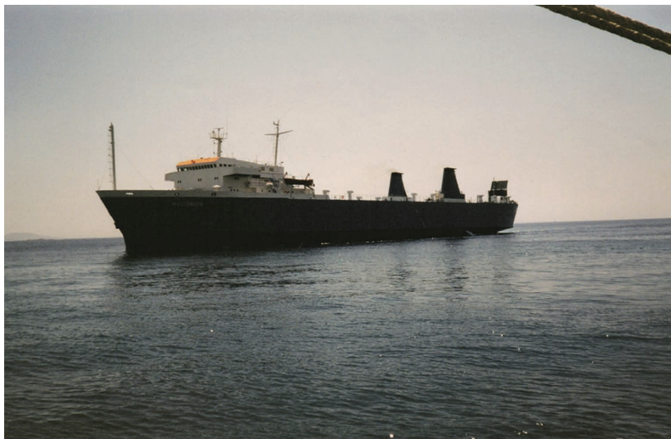
FIGURE 8.5 the MYKONOS modern Greek operated Roll on, Roll off ferry. Design features include all accommodation forward. A stern door/combined vehicle ramp right aft in the upright closed position when the vessel is at sea.
