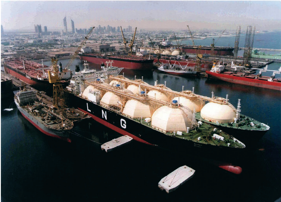
FIGURE 6.32 Two liquid natural gas carriers lay alongside each other, outside the Dubai dry dock complex. These dedicated ships are prominent for the conspicuous cargo domes covering the gas tanks.
