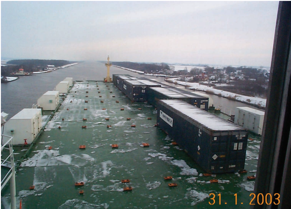
FIGURE 10.6 The steel fore deck of the Baltic Eide (IMO No. 8801917) fitted to receive containers overall, but seen above with a part load of containers, as its deck cargo, during a transit of the Kiel Canal.
