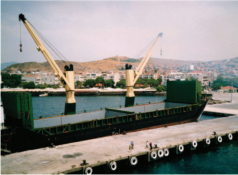
FIGURE 2.13 Open hatchway seen exposing the two cargo holds of the 'Scandi Spirit' (IMO No. 8817837) with the folding 'M' type hydraulic hatch covers in the fixed open position. The hatches are serviced by two port side pedestal cranes.
