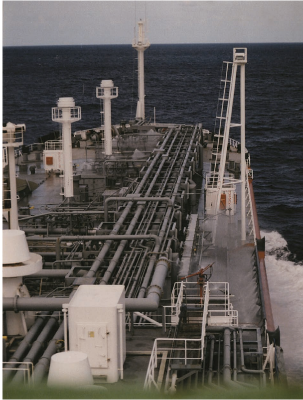
FIGURE 6.10 Typical example of the pipeline and ventilation arrangements (fore deck) of a medium-sized oil tanker seen in the seagoing environment.
