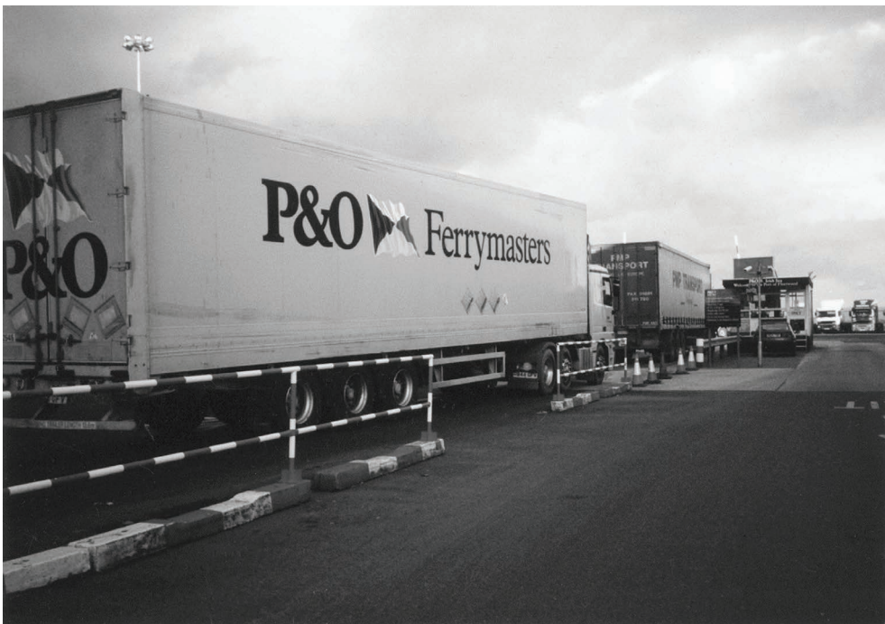
FIGURE 8.30 Ro-Ro mobile units entering the freight compound prior to customs clearance and redirection to the link span for loading on to the drive on ferry.
