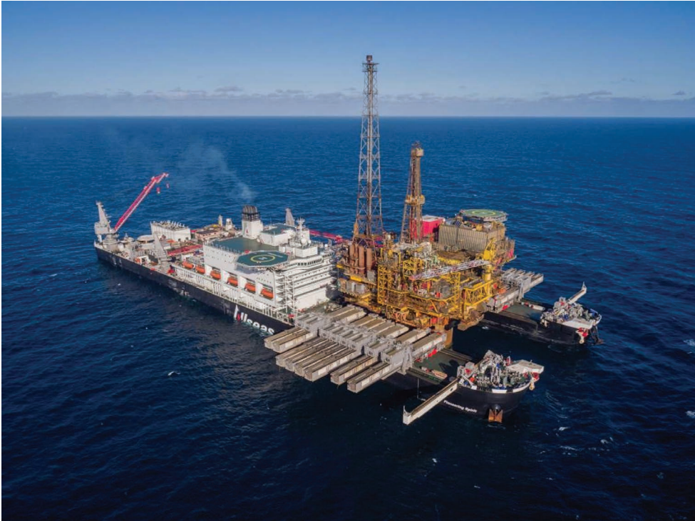
FIGURE 4.30 The world's currently largest ship Pioneering Spirit (IMO No. 9593505) has the equivalent deck space of six football pitches and has a lift capacity of 48,000 tons. In April 2017, the ship was engaged to lift the Brent Delta topside accommodation module, off the oil rig platform in the North Sea. The lift was 24,000 tons and was achieved in 12 hours by positioning the twin ballast hulls of the Pioneering Spirit under the rig and de-ballasting the ship to rise. (This lift holds the world's lifting record.)
