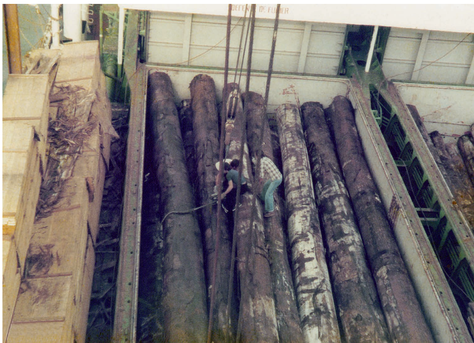
FIGURE 7.4 A cargo of heavy logs stowed under decks in twin hatches being discharged by multi-fold lifting purchase. Wire snotters are used to manoeuvre the logs to allow slings to be passed under, prior to discharging. Slings are often left in situ after loading to ease discharge, but not always. Sawn bundles of lumber are seen stowed at the hatch side as deck cargo.
