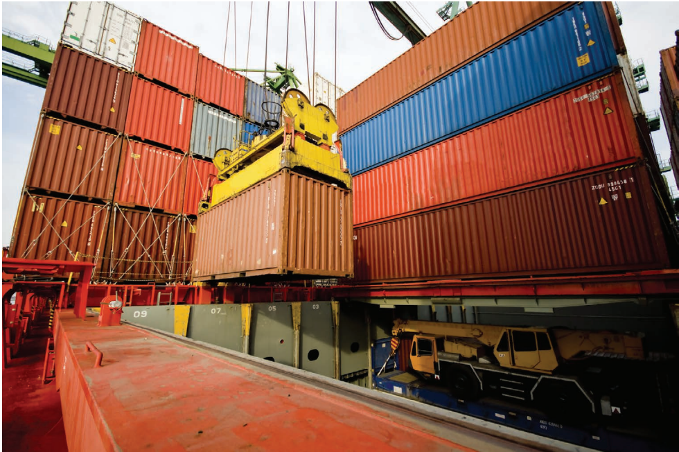
FIGURE 9.17 The container spreader beam operates secured to the gantry crane travelling the length of the gantry jib to lift the containers on and off the vessel. The corners of the spreader beam are fitted with hinged droppable guides to ensure the beam locks can accurately locate the container corner recesses. The beam is also used to lift off pontoon hatch covers but, when doing so, does not deploy the hinged guides.
