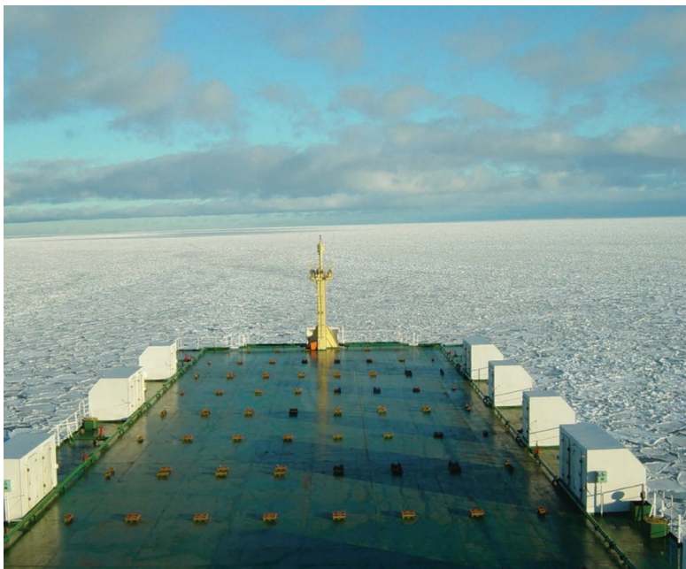
FIGURE 9.22 The exposed container forward cargo deck of the Baltic Eider (IMO No. 8801917) seen with the container deck stool securing points in uniform rows to form the basis of an even stow. The vessel is moving forward through 10/10ths light pancake ice in the Baltic Sea.
