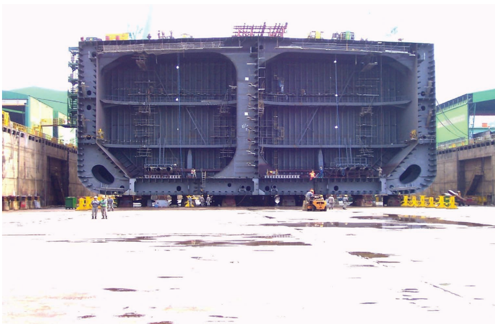
FIGURE 6.5 Athwartships cross-section of the modern double hull tanker seen at a late construction stage prior to assembly.
