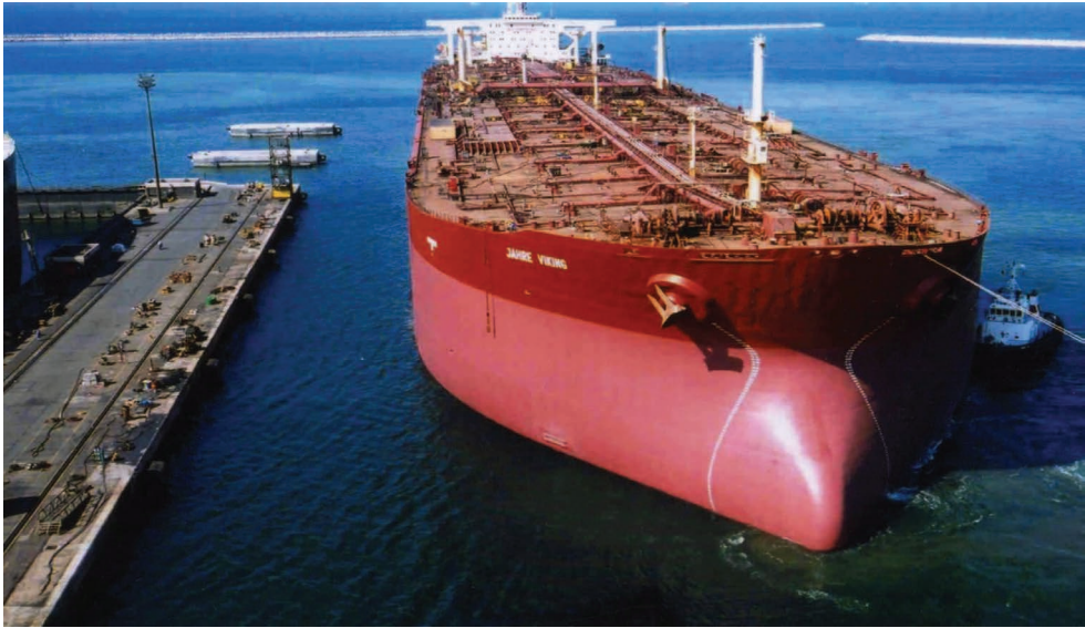
FIGURE 6.3 The Jahre Viking at 564,000 dwt (IMO No. 7381154) was the largest man-made transport in the world. It is seen manoeuvring with tugs off the Dubai Dry Dock. This vessel has been converted to a floating oil storage unit to prolong its active life.
