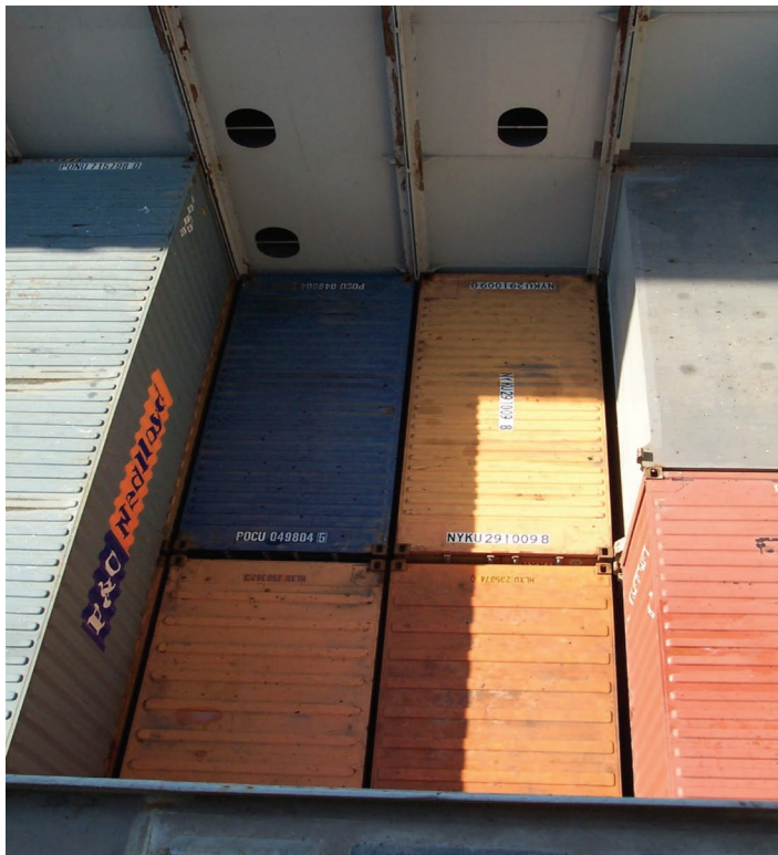
FIGURE 9.19 Container 'bay' (hatch) with part load containers lying in the cell guides of the lower hold cargo space.
