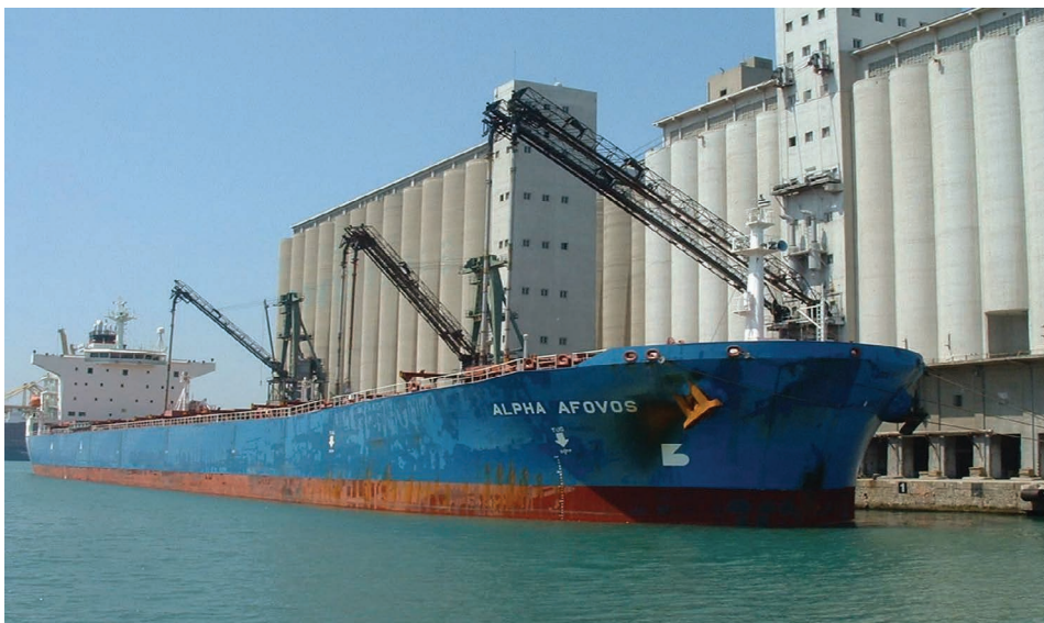
FIGURE 5.14 Bulk carrier Alpha Afovos (IMO No. 9221853) lies port side to the grain silos in Barcelona. The grain elevators are seen deployed into the ship's hold effecting discharge.
