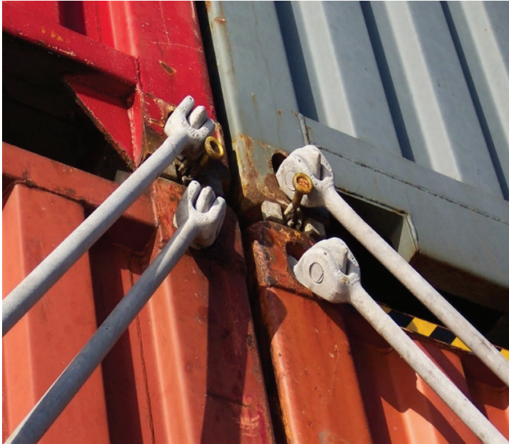
FIGURE 9.28 Container lashing bars, seen secured from the main deck to the first and second tier of deck containers.
