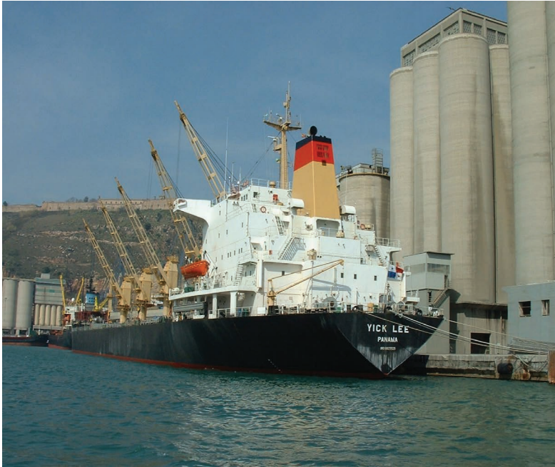
FIGURE 1.18 The bulk carrier 'Yick Lee' (IMO No. 8025525) seen starboard side to the grain berth, Barcelona, Spain. The ship has turned her deck cranes outboard to port to allow access for the suctions of the grain elevators to discharge a bulk cargo of grain.
