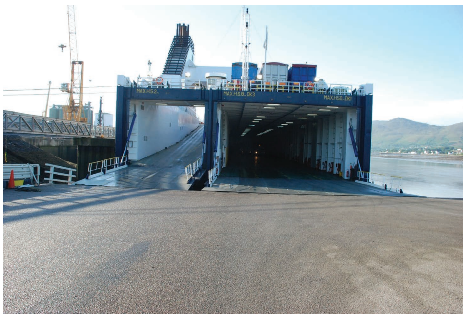
FIGURE 8.11 Example stern door/ramp access into the enclosed vehicle deck of a Ro-Ro ferry operating on the Irish Sea trade. Fixed ramp aspect seen on the port side of the vessel leads to the upper cargo deck where drop units have already been stowed.
