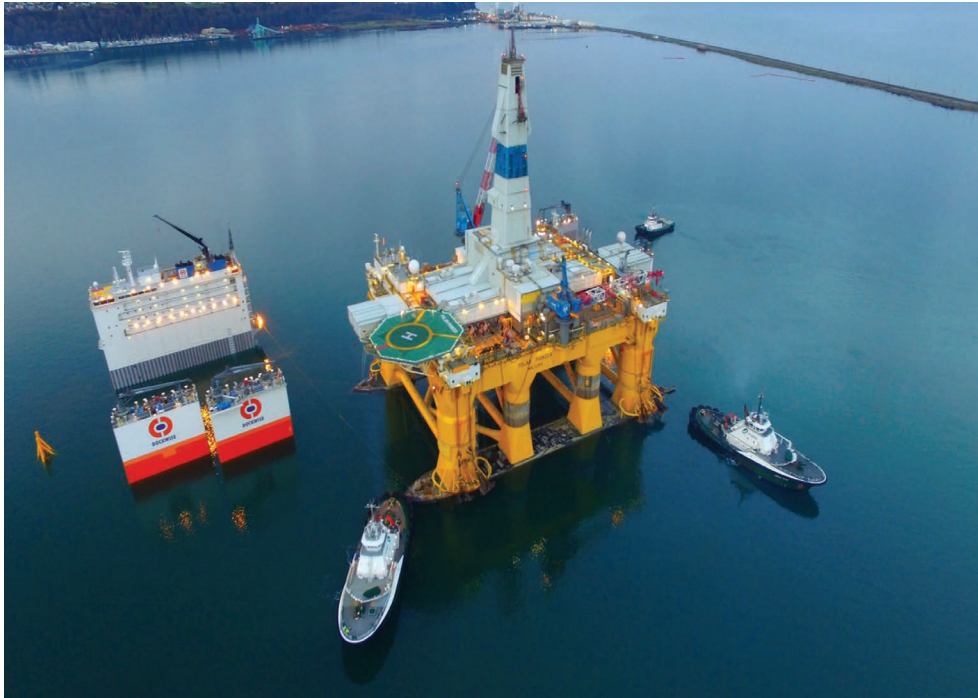
FIGURE 4.29 The offshore installation Polar Pioneer is seen being manoeuvred with tug assistance over the submersed platform deck of the semi-submersible Dockwise Vanguard .
