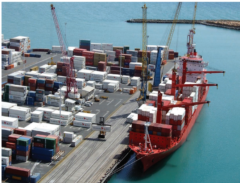
FIGURE 1.19 The 'Tasman Crusader' (IMO No. 9344667) renamed ( Cap Patton ) seen fitted with its own deck container cranes working containers by shore side cranes while starboard side to, in Napier, New Zealand. The ships own deck cranes are turned outboard to allow working space for cargo movement.
