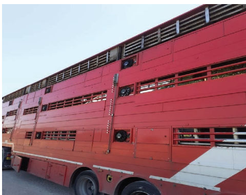
FIGURE 7.13 Livestock transporter. Typical road transporter for 'Pigs' allows three tier carriage with roof and side ventilation also electrically driven fans and drinking wells to all three levels.
