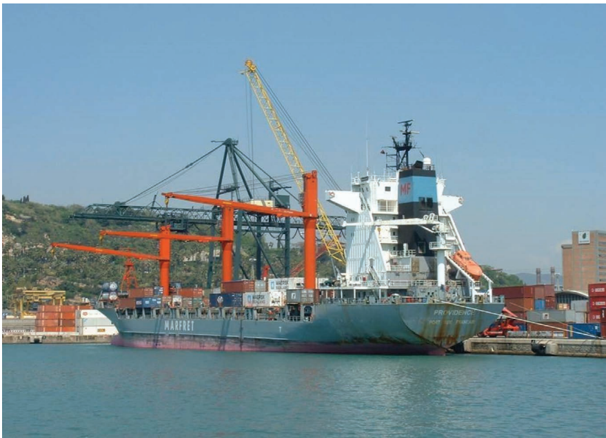
FIGURE 9.30 A single gantry crane and a mobile dockside crane work the container cargo of the feeder container vessel Providence (IMO No. 9080417). The ship's own container cranes are seen turned outboard to facilitate the shoreside loading systems in the port of Barcelona.
