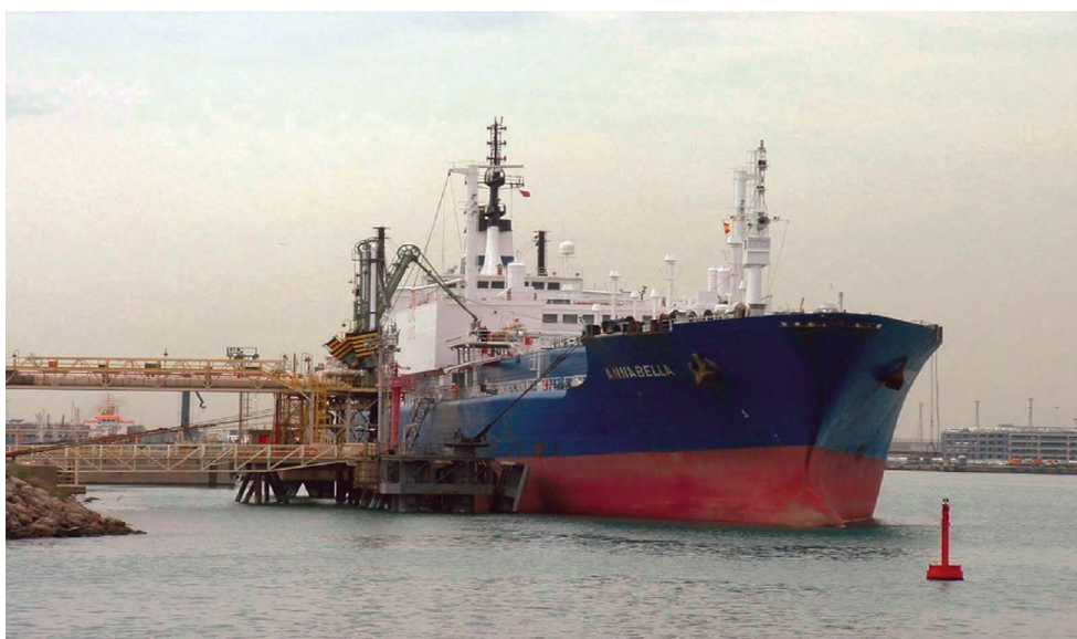
FIGURE 6.41 The Monrovia LPG gas tanker Annabella (IMO No. 9250684) seen starboard side to the gas terminal in Barcelona while engaged in gas cargo operations.
