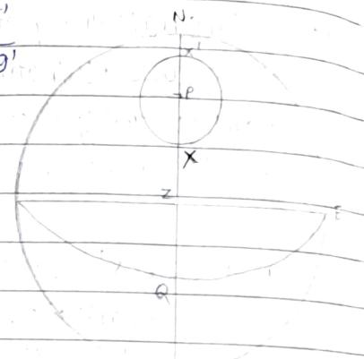
$$\text{Declination (QX)} = 90^\circ - \text{Polar distance (PX or PX')}$$
